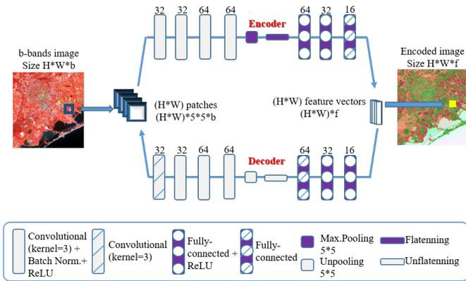
Fig. 1: Convolutional autoencoder with fully-connected layers.
